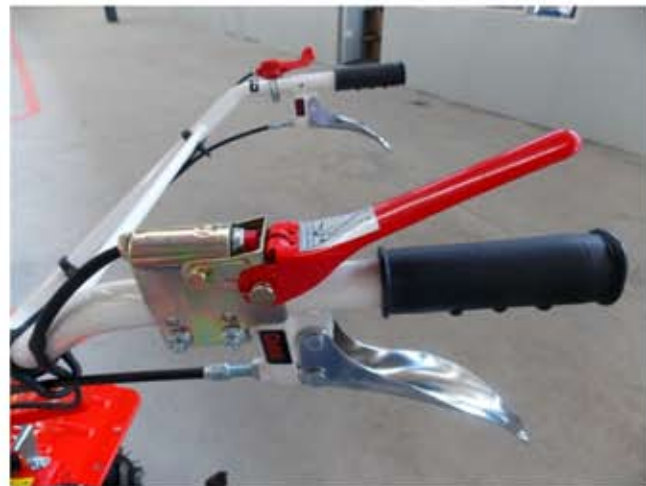
Metal handlebar for clutch handle, emergency stop handle, and reverse handle
