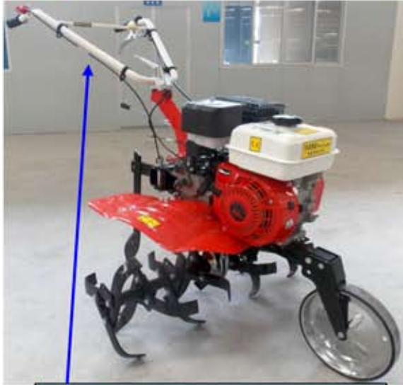
U shape handlebar, 360° horizontally adjustable
