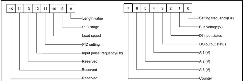
If the above parameters need to be displayed at the time of stop, it can set their corresponding positions to 1 and then convert this binary number into decimal number and set it to P7.05.
