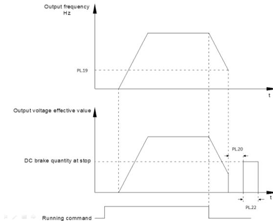
DC brake schematic diagram
