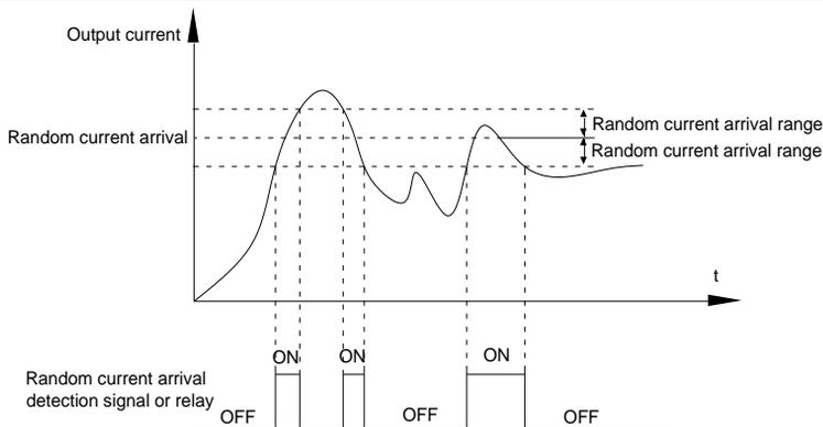
Fig.5-23 Random current arrival detection schematic diagram
