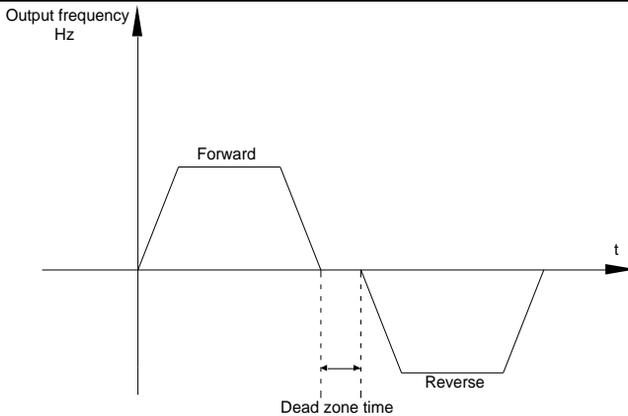
Fig.5-15 Rotation dead zone time schematic diagram
