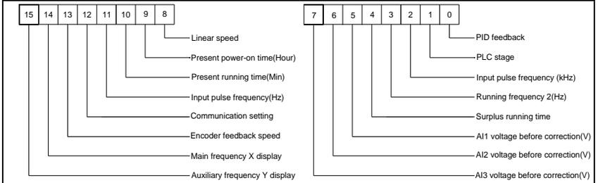
If the above parameters need to be displayed during the operation, users can set their corresponding positions to 1 and then convert this binary number into decimal number and set it to P7.04.
