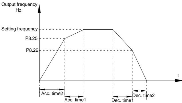
Fig.5-19 Acc./dec. Time switching schematic diagram
