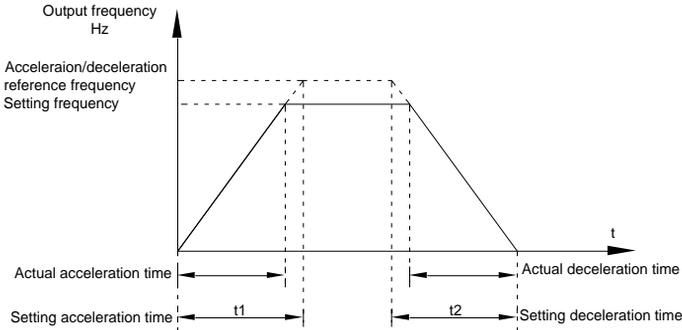
Acceleration/deceleration time schematic diagram
