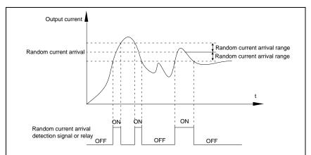
Fig.5-23 Random current arrival detection schematic diagram
