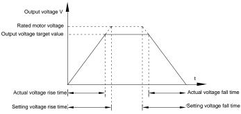
Fig. 5-5 VF separation schematic diagram
