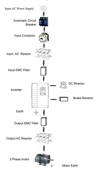
Fig.3-1 Connection diagram of the product and peripheral devices
