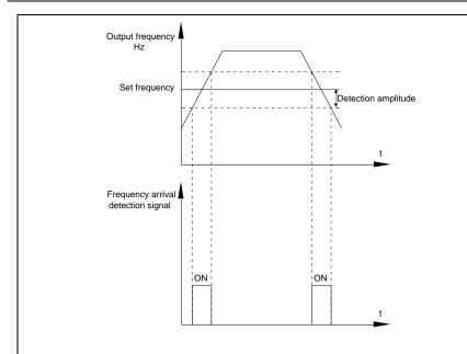
Fig.5-17 Frequency arrival detection amplitude schematic diagram
