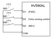
Fig. 5-8 Three-line control mode 1
