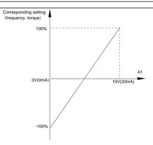
Fig. 5-10 Relationship between analog input and setup value
