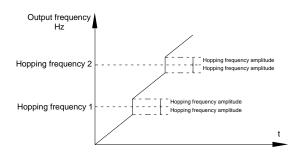
Fig.5-18 Acc./dec. hopping frequency validity schematic diagram
