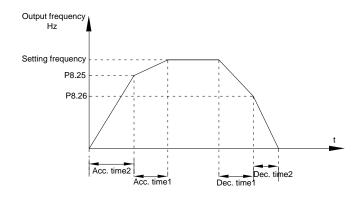
Fig.5-19 Acc./dec. Time switching schematic diagram
