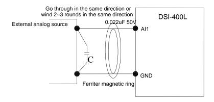
Fig.2-6.2 Analog input terminal processing wiring diagram
