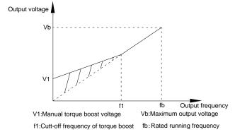
Fig. 5-3 Manual torque boost schematic diagram
