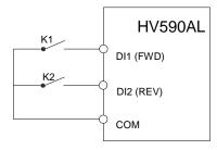
Fig. 5-7 Two-line control mode 2
