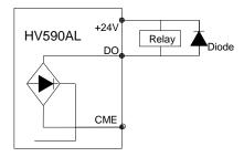
Fig. 2-6.5 Digtal output terminal wiring diagram
