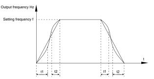
S-curve acceleration/deceleration schematicdiagram A
