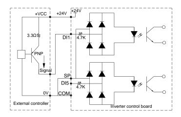
Fig. 2-6.4 Source wiring mode
