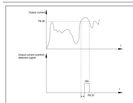
Fig.5-22 Output current over limit detection schematic diagram
