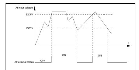
Fig.5-31AI terminal valid state schematic diagram
