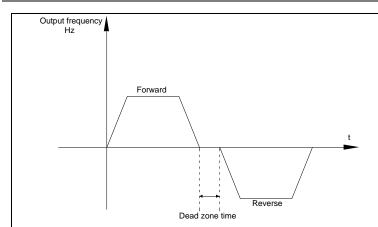
Fig.5-15Rotation dead zone time schematic diagram
