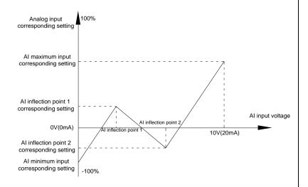
Fig.5-32Curve4 and curve 5 schematic diagram
