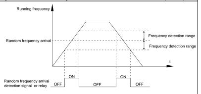
Fig.5-20 Random frequency arrival detection schematic diagram
