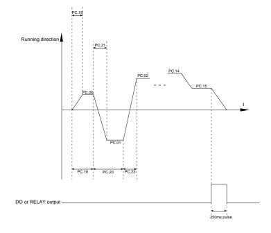
Fig.5-30Simple PLC schematic diagram
