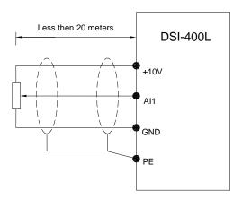
Fig. 2-6.1 Analog input terminal wiring diagram
