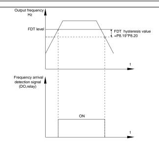
Fig.5-16 FDT level schematic diagram
