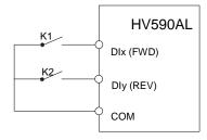
Fig. 5-6 Two-line control mode 1
