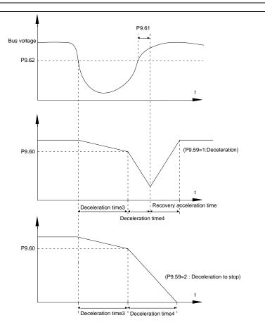
Fig.5-24 Transient stop action schematic diagram
