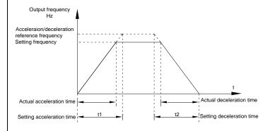
Acceleration/decelerationtime schematic diagram
