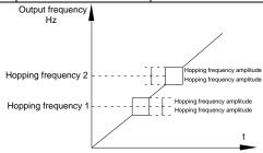
Fig.5-14Skip frequency schematic diagram
