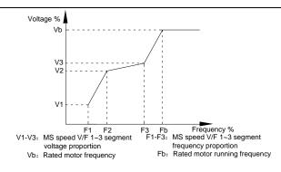
Fig. 5-4 Multi-point V/F curve setup schematic diagram
